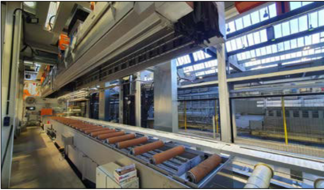
Figure 4. The new quench provides precise cooling of the profiles to meet strict automotive and other industry standards.
